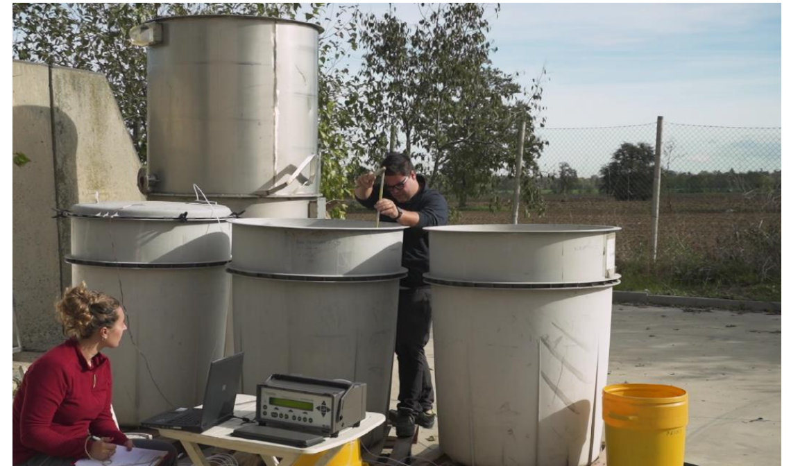
Emission monitoring from storage for 60 days by Static chamber method and photoacoustic multi gas analyzer (INNOVA 1412) (Denmead, 1979; Hornig et al, 1999; Pedersen et al., 2001)
