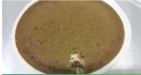
Current stage of struvite refinement, struvite-rich precipitate
