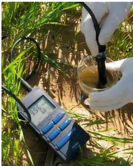
Field Use of a Manual Conductivity Meter to Determine Slurry Application Rates Based on Nutrient Content
