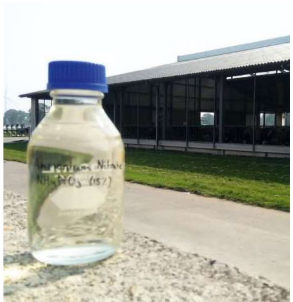
Ammonium nitrate recovered from manure stripping and scrubbing process
