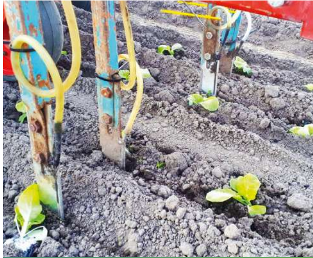
Application of ammonium salts to grass and vegetable crops through injection to reduce ammonia emissions
