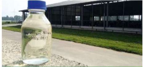
Ammonium salts are produced from the Stripping-scrubbing process
