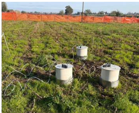
On-site measurement of ammonia emissions by Wind tunnel technique (left) and GHG emissions by static Chamber (right)
